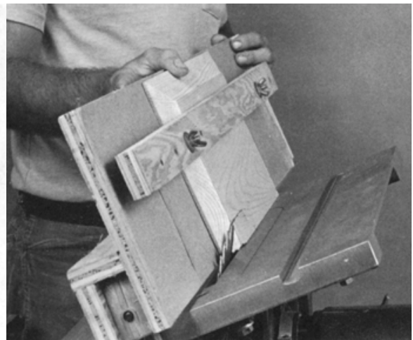
Figure 4-23. To use the raised panel fixture, tilt the table 5 degrees to 15 degrees. Place your stock in the fixture, secure the mounting screws as close to the panel as possible.
